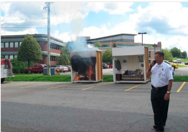
**Photo 13:** For training purposes, the fire sprinkler in the room was opened manually. Chief Caravaso explains to the RAs how effectively and quickly fire sprinklers control a room fire. After only a few seconds of sprinkler operation, the fire is knocked down.
