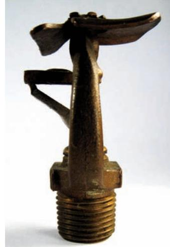
*Photo 10: 1956 Rockwood sidewall 165°F, 1/2 inch K=5.6 sprinkler. This sidewall is designed to be installed in the upright position.*
