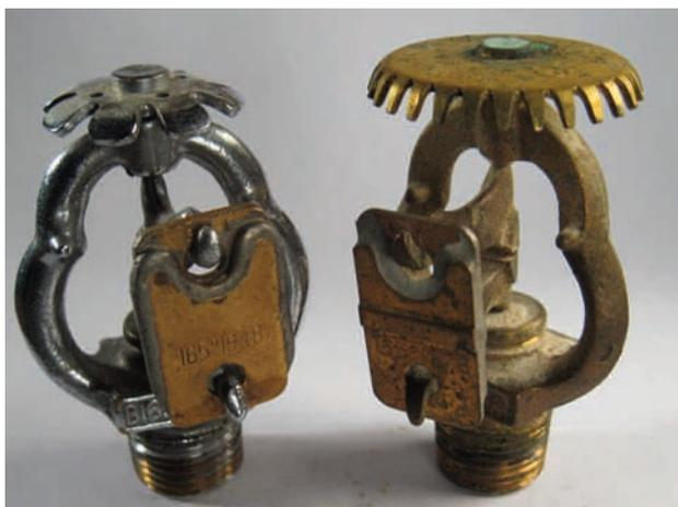
**Photo 8: 1946 Hodgeman Model B chrome 165°F (left) and 1976 Model D SSU 165°F (right) heads. Hodgeman heads were readily identifiable by their distinctive frame design.**
