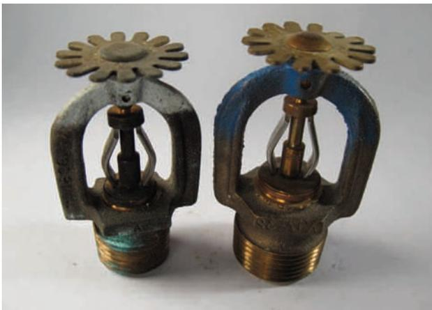
*Photo 9: 1985 Central, Model A, SSP, intermediate temperature 212 °F, 1/2 inch K=5.6 (left) and 1978 Central, Model A, SSP, high temperature 286 °F, 17/32 inch K=8.0 (right) sprinkler heads. Notice the color coding, white for intermediate and blue for high temperature. Also, the larger orifice sprinkler head has 3/4-inch NPT threads to allow for more waterflow through the head. The thread size is also a quick identifier that this is a k=8.0 large orifice sprinkler.*
