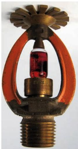
**Photo 6: (right) 1947 Automatic Model A, 286 °F sprinkler. This head is used in areas where the ambient temperature may reach up to approximately 230 °F. It may be used near heater units to prevent accidental operation. They are also used over storage occupancies.**
