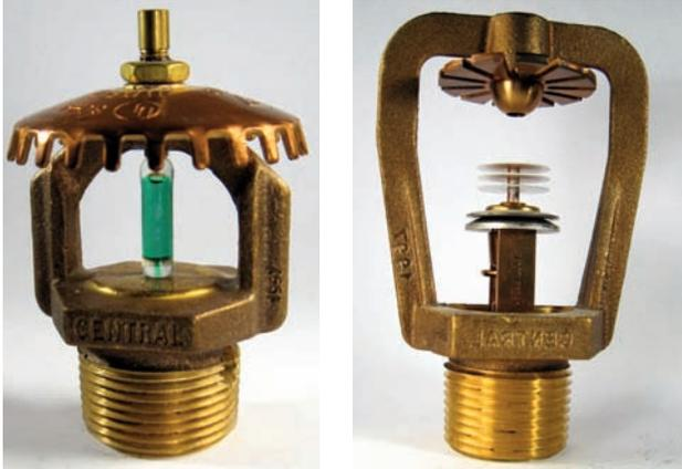
*Photo 12: (left) 1997 Central K-17-231 CMSA upright 200 °F sprinkler head. This head is a special application for storage occupancies. This head has a K factor of 17. Notice the pintle on the top of the deflector, which denotes a special or nonstandard sprinkler head.*
