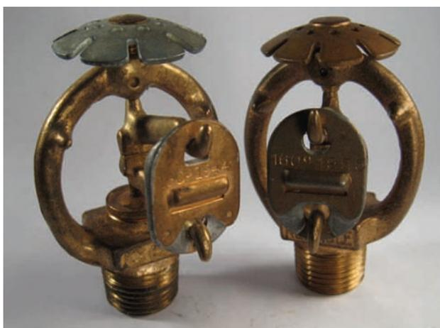
**Photo 7: 1944 and 1955 Reliable Model C, 160°F sprinklers. The deflectors on these heads are slightly larger than some other sprinkler heads of the era and compensated by drilling holes in the top of the deflector. During World War II, brass was at a premium, and the deflector was manufactured from a different metal.**
