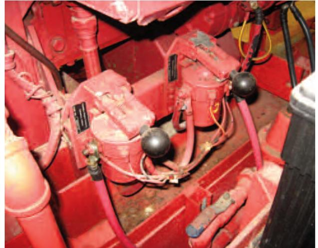
**Photo 11: Battery contactor levers located on the side of a diesel engine.**
